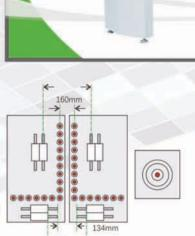
Optimized drill layout and collinear design of two drilling blocks 'vertical drills increase the efficiency at lease by 30%. Mini part up to 200\*30mm, two panels can be proceed together.
